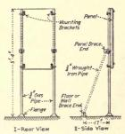
Fig. 208.—Wrought-iron pipe support for small panel.
